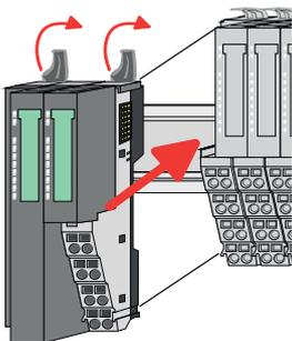
**7.** To mount the bus coupler put it to the left periphery module and push it, guided by the stripes, to the mounting rail.
