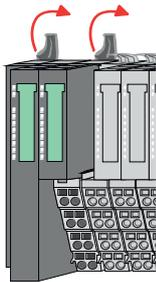
**4.** Turn all the locking lever of the bus coupler to be exchanged upwards.
