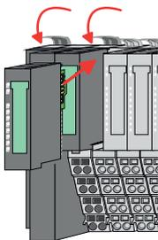
**9.** Plug again the electronic module, which you have removed before.
