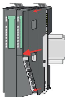
1. Before mounting the peripheral modules you have to remove the bus cover at the right side of the bus coupler by pulling it forward. Keep the cover for later mounting.
