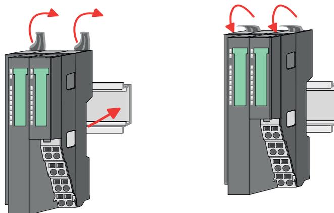
2. Turn the locking lever upwards, place the bus coupler at the mounting rail and turn the lever downward.
