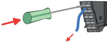
The wire is to be removed by means of a screwdriver with 2.5mm blade width.
