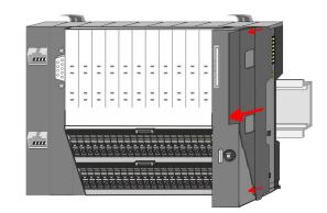
**1.** Before mounting the periphery modules you have to remove the bus cover at the right side of the CPU by pulling it forward. Keep the cover for later mounting.
