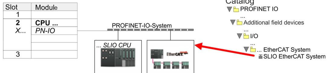
1. Navigate in the hardware catalog to the directory 'PROFINET IO → Additional field devices → I/O → ... EtherCAT System' and connect the IO device 'SLIO EtherCAT System' to your PROFINET system.
