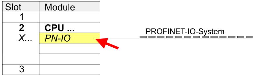
6. → Create with [New] a new sub net and assign valid address data.
