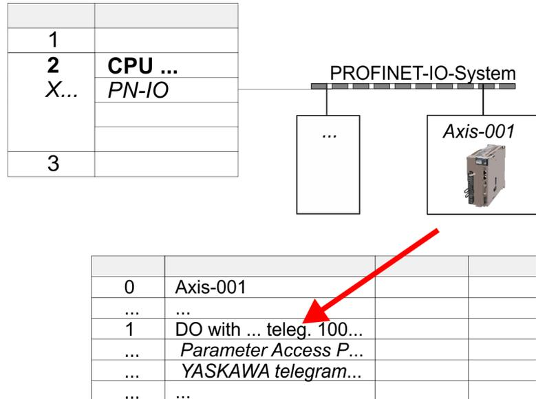
5. In the hardware catalog, expand the *Sigma-5* PROFINET drive 'SGDV-xxxxE1...' to show its components and drag&drop the component 'DO with YASKAWA teleg. 100...' to slot 1 of the *Sigma-5* PROFINET drive.
