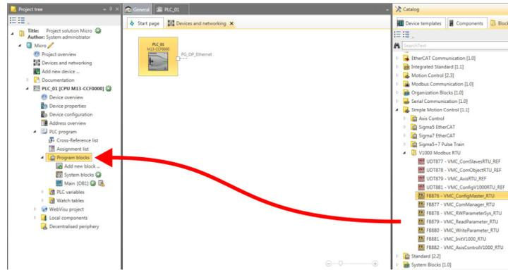
2. In the 'Catalog' at 'Blocks → Simple Motion Control' open the collection 'V1000 Modbus RTU' and drag and drop the following blocks into 'Program blocks' of the Project tree:
