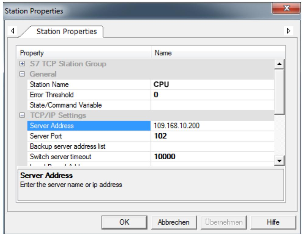
7. → Negate the query for importing variables from the PLC database and close the 'S7 TCP' dialog with [OK].
