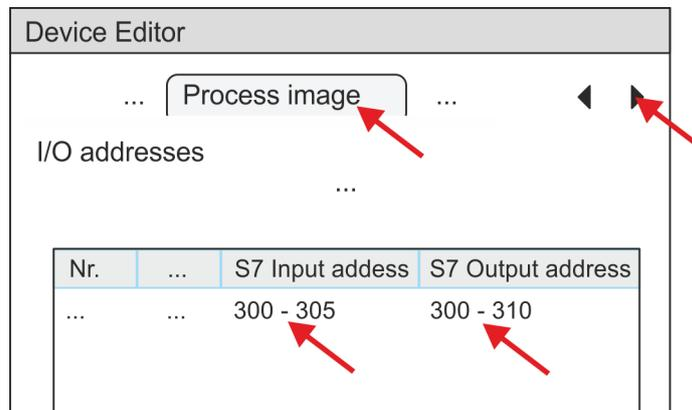
16. By closing the *SPEED7 EtherCAT Manager* with [X] the configuration is taken to the project. You can always edit your EtherCAT configuration in the *SPEED7 EtherCAT Manager*, since the configuration is stored in your project.
