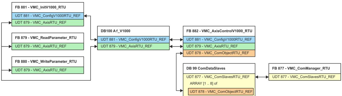
With the exception of blocks DB 99 and FB 877, you must create the blocks listed below for each connected inverter drive:
