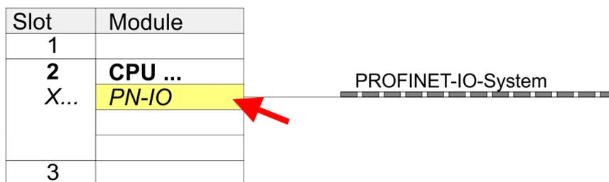
3. ➔ Create with [New] a new sub net and assign valid address data
