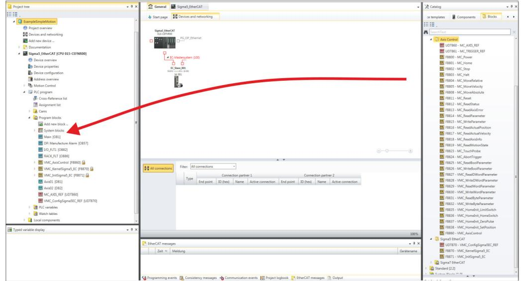
➔ In the 'Catalog', open the 'Simple Motion Control' library at 'Blocks' and drag and drop the following blocks into 'Program blocks' of the Project tree:
