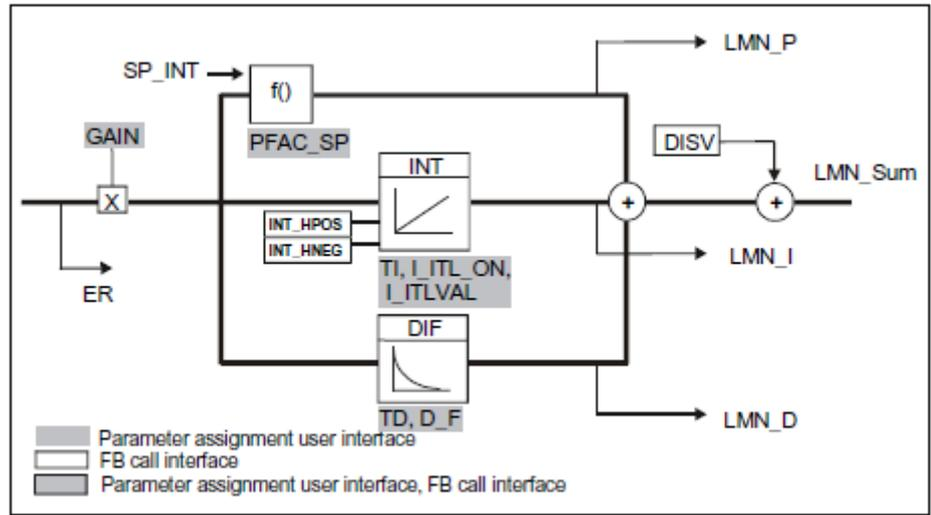
**PID Algorithm (GAIN, TI, TD, D\_F)**
