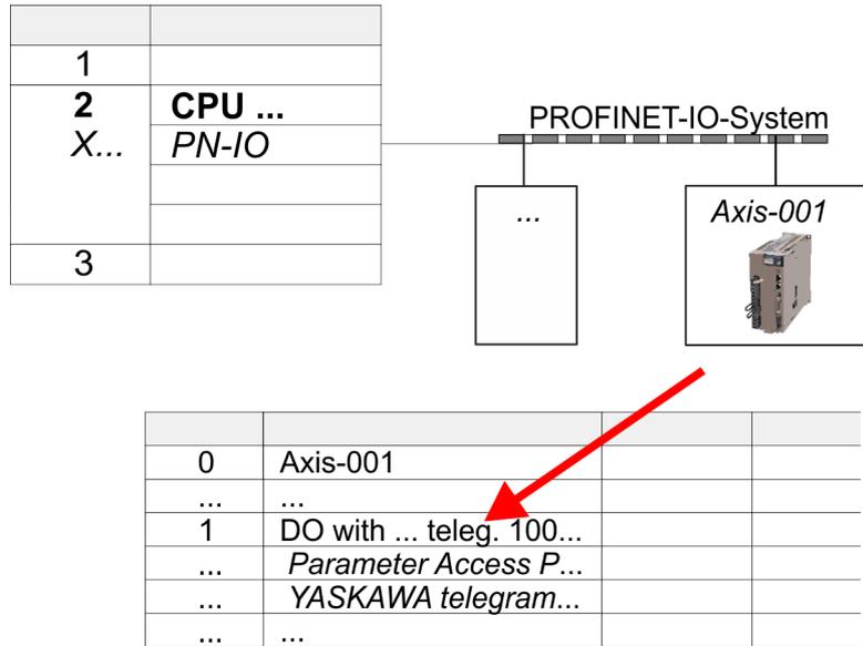
5. In the hardware catalog, expand the *Sigma-7* PROFINET drive 'SGD7S-xxxAC0xxxx' to show its components and drag&drop the component 'DO with YASKAWA teleg. 100...' to slot 1 of the *Sigma-7* PROFINET drive.
