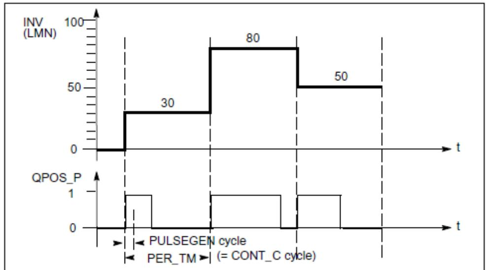
An input variable of 30% and 10 FB PULSGEN calls per *PER\_TM* means the following:
