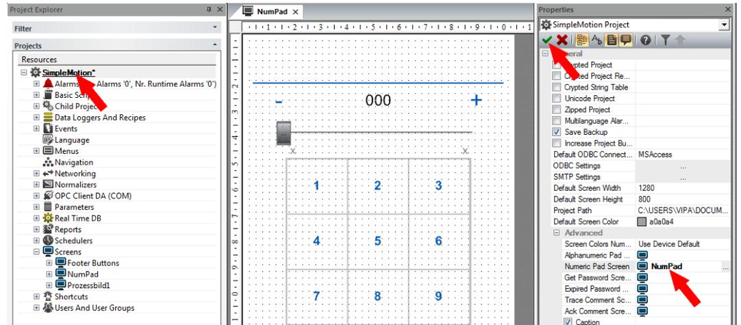
8. For optical adjustment click at 'Resourcen > SimpleMotion > Screens > NumPad > Drawing Objects > Touchpad\_Num' at 'Schieberegler' (slide control) and select 'Context menu → Properties'. Expand the 'Style' part and disable 'Show Bar'.
