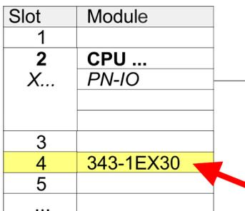
1. → Place for the Ethernet PG/OP channel at slot 4 the Siemens CP 343-1 (SIMATIC 300 \ CP 300 \ Industrial Ethernet \ CP 343-1 \ 6GK7 343-1EX30 0XE0 V3.0).
