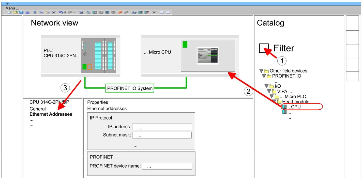
5. ➔ Select in the *Network view* the IO device such as '*... MICRO PLC*' and switch to the *Device overview*.
