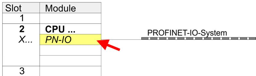
8. Create with [New] a new sub net and assign valid address data.
