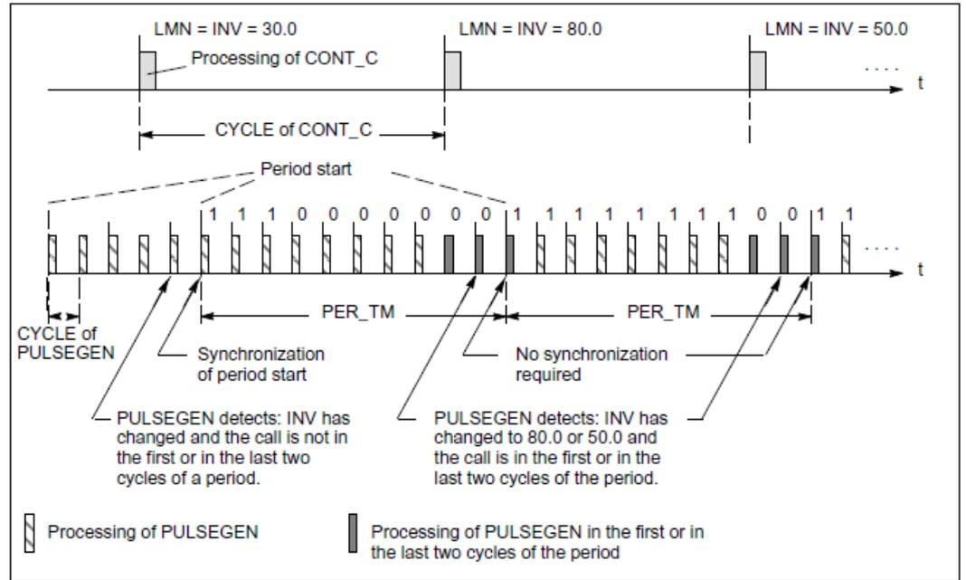
The automatic synchronization can be disabled at the SYN\_ON input (= FALSE).
