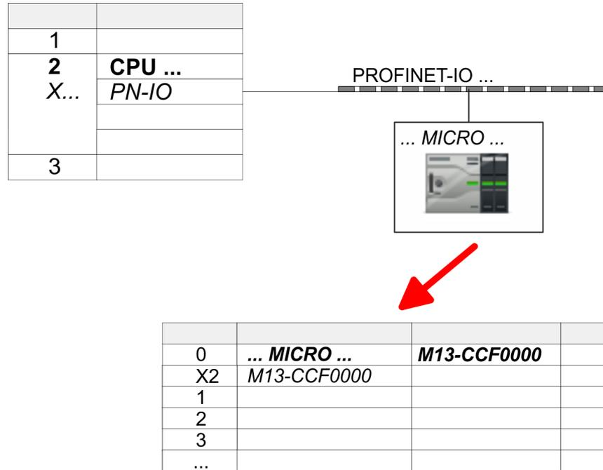
6. ➔ Navigate in the hardware catalog to the directory 'PROFINET IO → Additional field devices → I/O' and connect e.g. for the System MICRO the IO device 'M13-CCF0000' to your PROFINET system.
