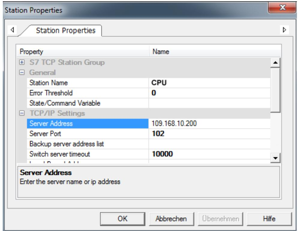
13. ➤ Negate the query for importing variables from the PLC database and close the 'S7TCP' dialog with [OK].
