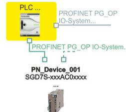
➔ The *Sigma-7* drive is connected to your PROFINET IO controller.
