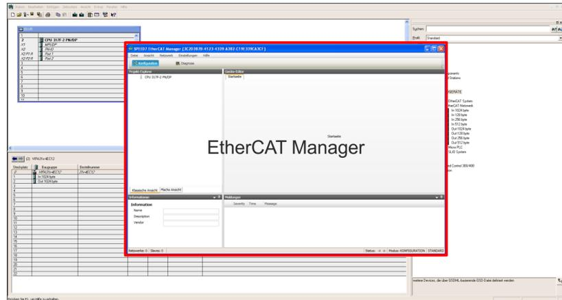
2. ➤ For the inverter drive to be configured in the *SPEED7 EtherCAT Manager*, the corresponding ESI file must be installed. The ESI file for the inverter drive can be found under [www.yaskawa.eu.com](http://www.yaskawa.eu.com) in the 'Download Center'. Download the according ESI file for your drive. Unzip this if necessary.
