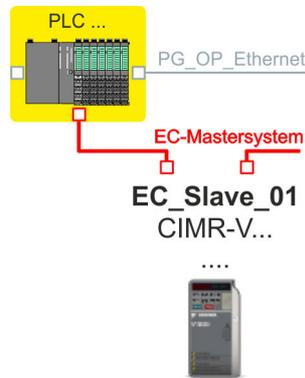
➔ The inverter drive is connected to your EC-Mastersystem.
